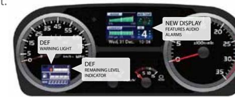
From a driver's standpoint, it does not get any easier; simply refill the DEF tank at normal refill intervals. Filling your truck with DEF is not much different than re-fueling with diesel; however the usage ratio is significantly less. The DEF dose rate is on average 1-2% DEF for each gallon of fuel consumed. The DEF tank on a Hino truck will accommodate 4.7 gallons of DEF which allows the vehicle to travel as many as 8,000 miles between DEF tank refills (on highway usage).
