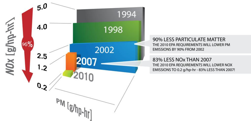
SCR is the best choice for meeting the EPA10 regulations for many reasons. It is a proven technology with more than 600,000 vehicles globally currently operating with SCR. Also, SCR is a long term solution with over 30 years of technology advancements. Another benefit of SCR is that it enables the engine to operate under optimized combustion conditions and does not require any complex engine subsystem modifications.
